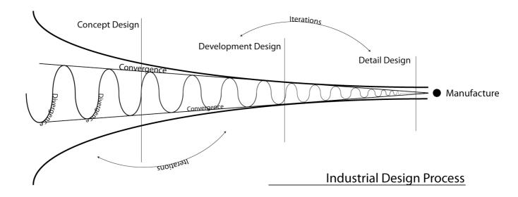
Fig 1. Generic model of industrial design process
