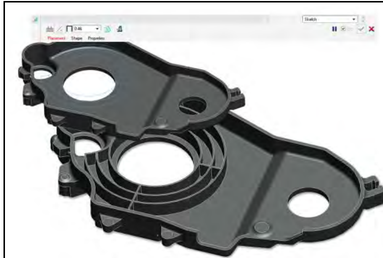
Figure 2.27 Shelled CAD model for use in support of engineering
