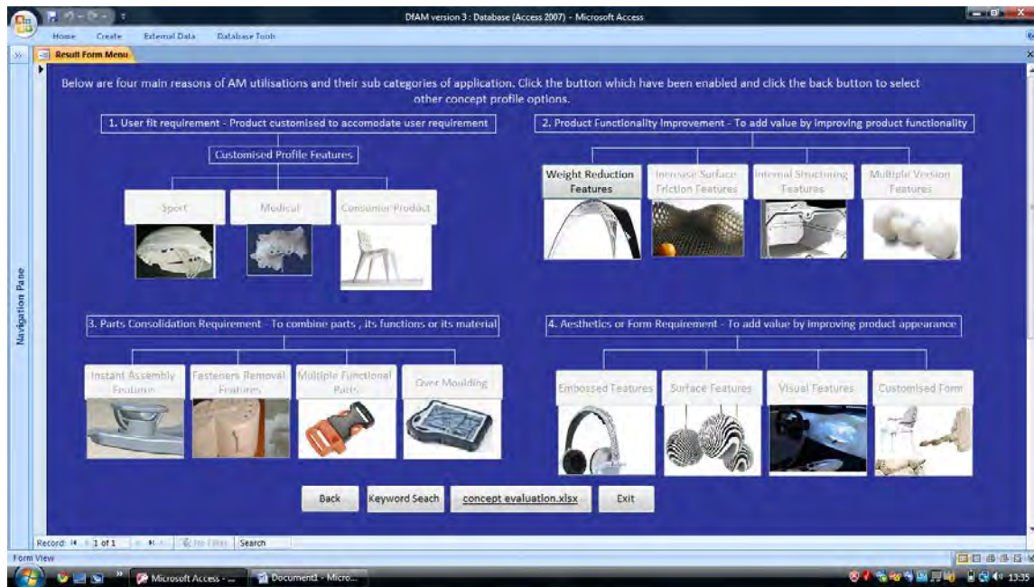
Figure 5 The DfAM repository, screen showing reasons for the use of additive manufacture
