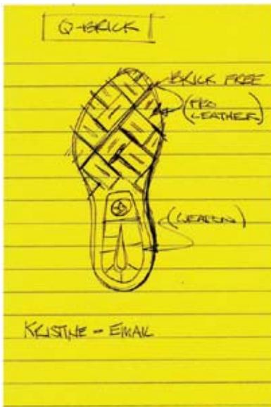
THUMBNAIL SKETCH: DONE 'ON THE FLY' TO QUICKLY COMMUNICATE DESIGN THINKING
